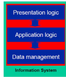
Figure 7.16: A conventional GIS contains all components inside the same system. A WebGIS separates the management, application and presentation part, and makes it accessible to a client. (Source: B. Köbben, ITC).
