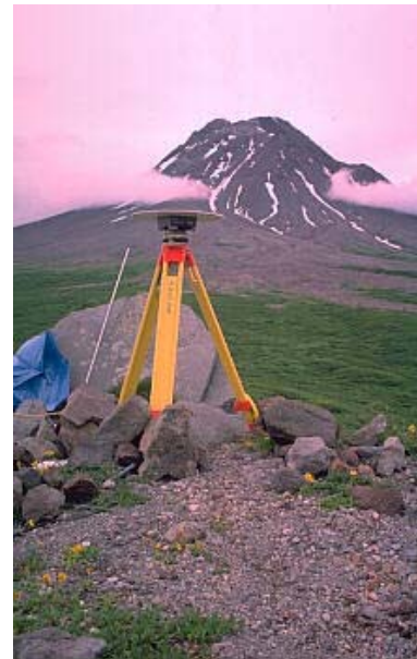
Figure 3.V.11: Differential GPS deployed at a volcano.
